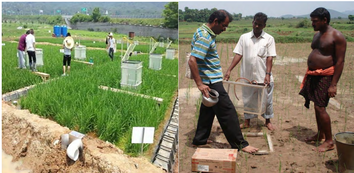
Test plots shown on left at Kangwon National University in Korea set up to measure and compare GHG emissions from SRI and conventional management of rice cropping. On right, setting up measurement instruments in a farmer's SRI field in Orissa state of India, under an SRI program managed by the Centre for World Solidarity there.
