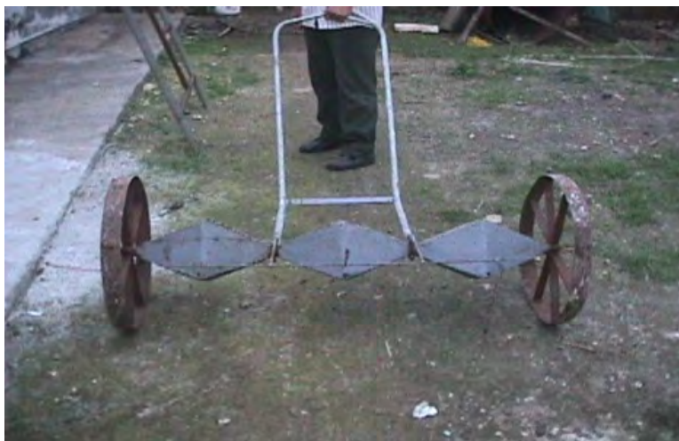
Three-row direct-seeder fabricated by Cuban farmer Luis Romero for 40x40 cm SRI spacing. This implement was not successful because this spacing was too wide, and weeds became too dominant. His neighbor built an ox-drawn 12-row seeder; but it also was not effective because it proved to be too awkward to be managed with oxen.
