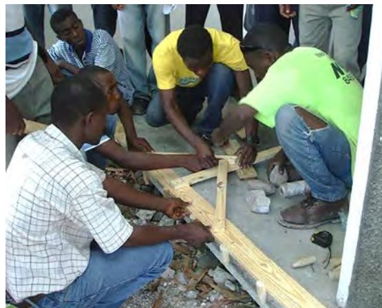
Young farmers in Haiti making a marker (rayonneur) out of wood to be able to mark their fields for transplanting SRI seedlings at 25 x 25 cm spacing.
