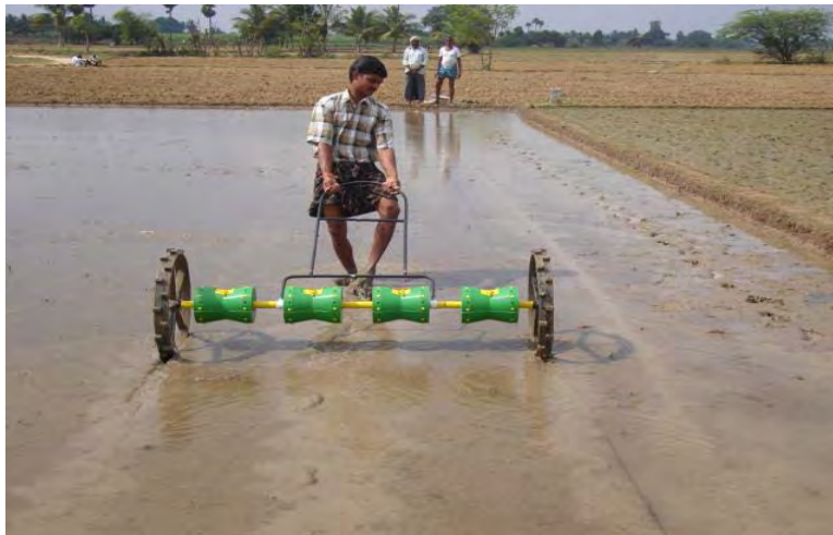
Drum seeder for direct-seeding SRI, developed at the RASS-Acharya Ranga KVK In Tirupati, Andhra Pradesh state of India (Hussain Reddy et al. 2011).
