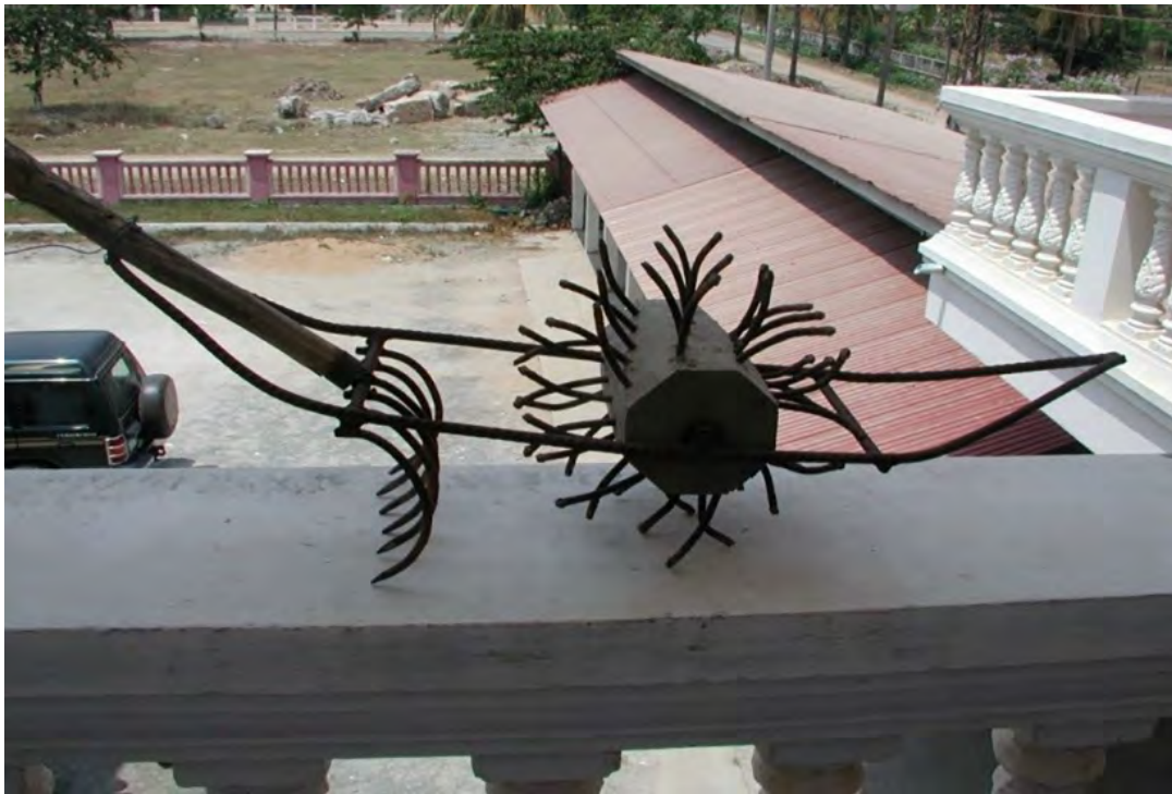
Weeder built by Nong Sovann, a farmer in Kandol village in Kampong Speu province of Cambodia. The materials cost him $3.60 -- for the large nails (that were driven into a wooden axle), the welding of iron rods, and adding a rake on the handle behind for better soil aeration. Nong estimated that this implement added at least $20 of value to the rice production from his very small field. See pages 9-10 of: http://sri.cals.cornell.edu/countries/cambodia/camphiltrpt305.pdf .
