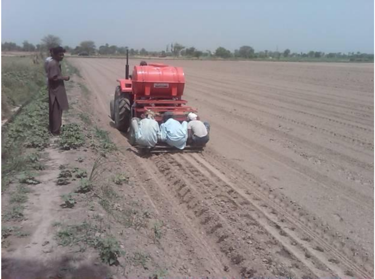
#9: Transplanting machine straddling raised bed, with water tank to provide initial water supply
