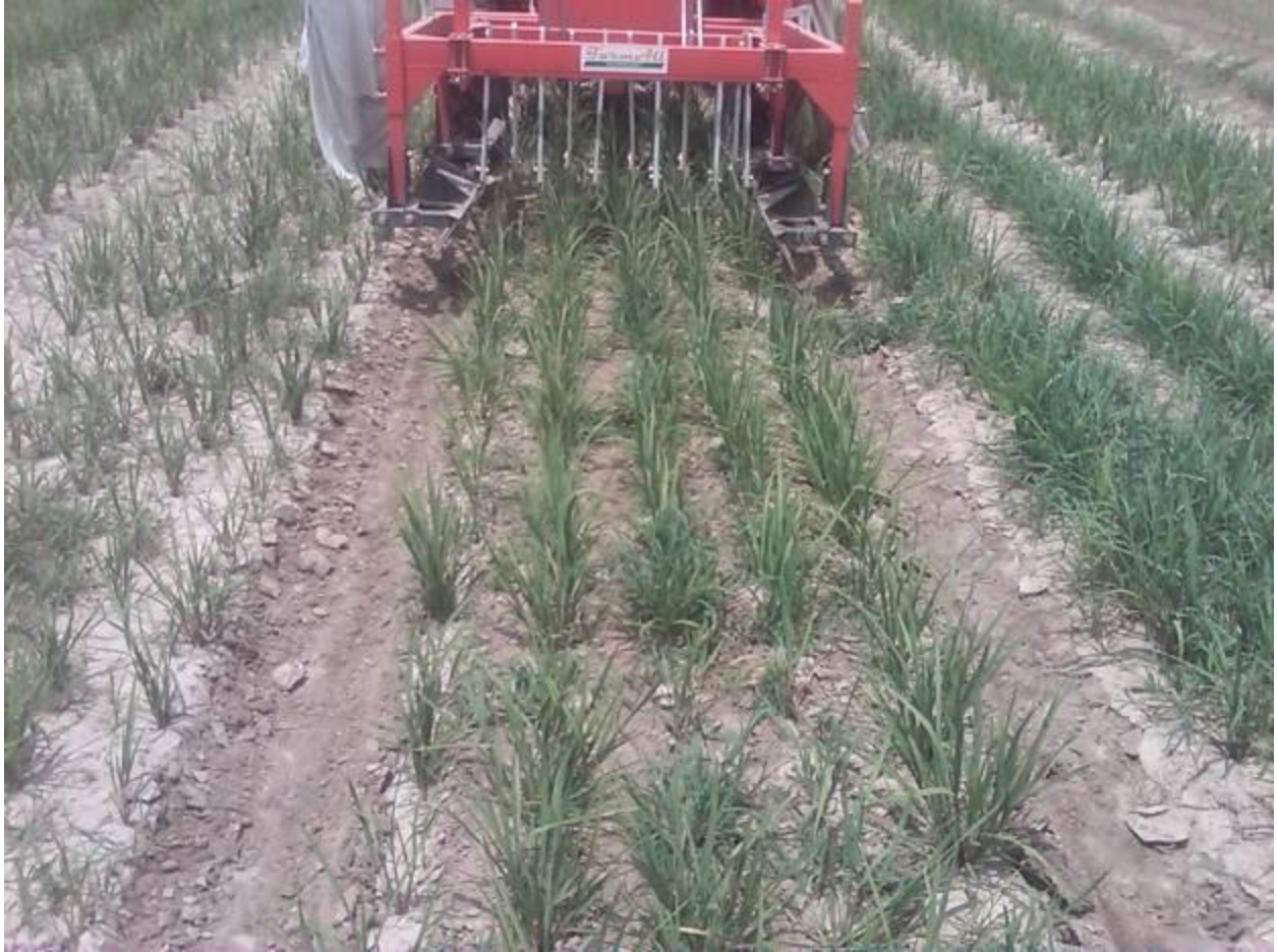
#12: Mechanical weeder, driving down the furrows, to weed between rows of rice plants
