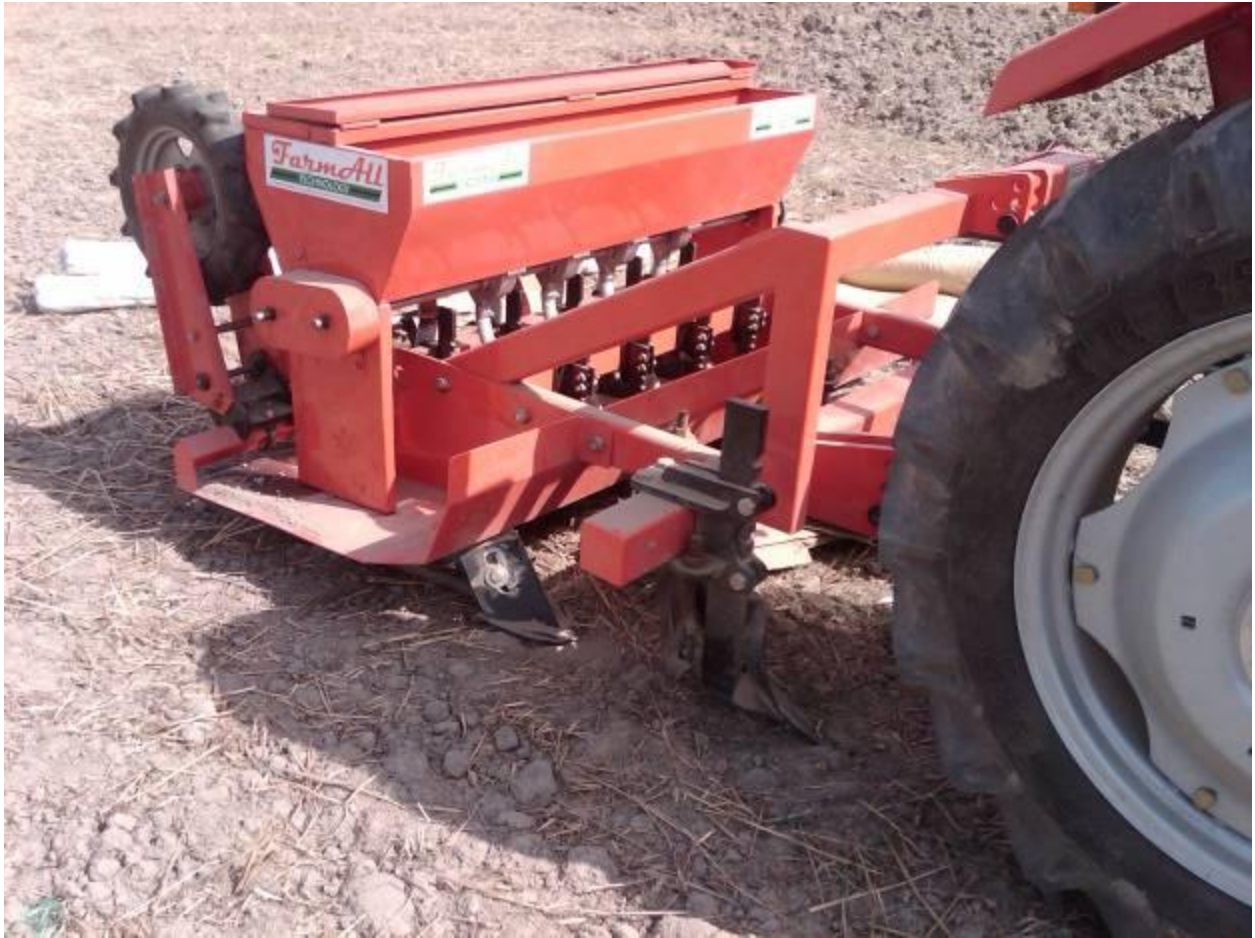
#4: Raisedbed maker with compost and fertilizer applicator
