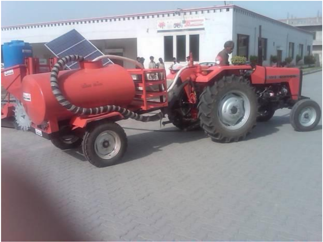
#6: Water bowser for supplying water to transplanting machine
