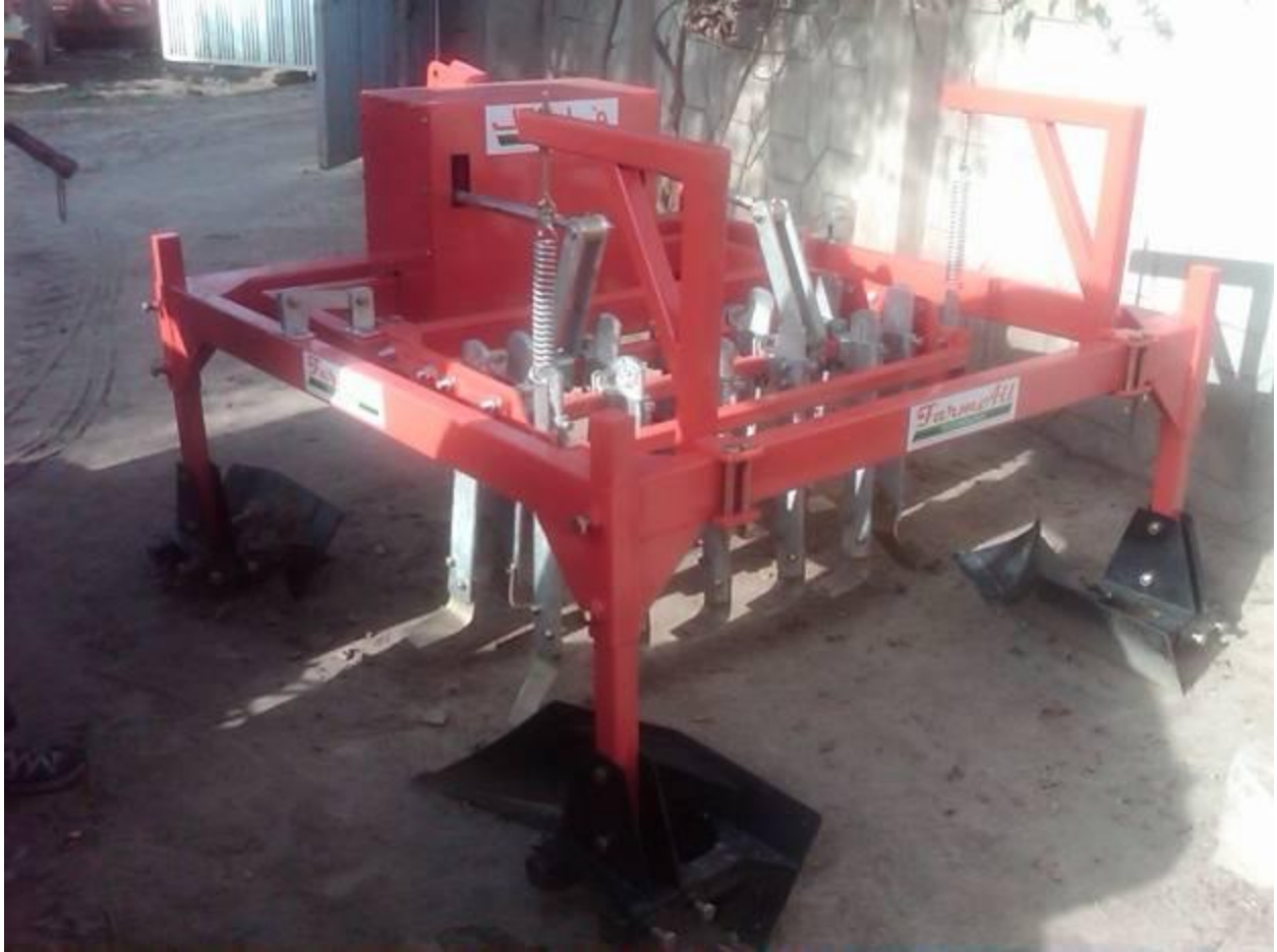
#11: Mechanical weeder designed for inter-cultivation between rows 9 inches apart (22.5 cm)
