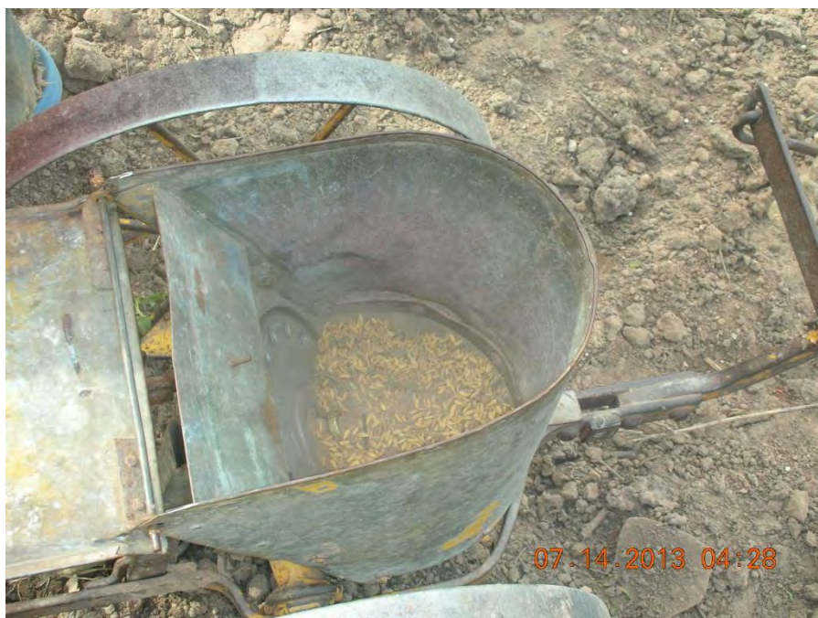
Figure 18: Animal traction seeder hopper attachment. Rice seed mixed with soil to reduce within-row plant density when seeding with a disc designed for corn. Photo by Lorraine Perricone – Dazzo
